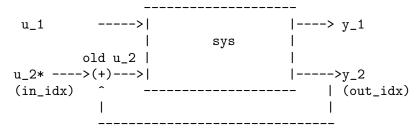
The input that has the summing junction added to it has an \* added to the end of the input name.
