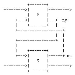
If ny and nu "consume" all inputs and outputs of K then the result is a lower fractional transformation. If ny and nu "consume" all inputs and outputs of P then the result is an upper fractional transformation.
