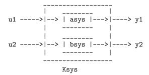
The function also rearranges the internal state-space realization of sys so that the continuous states come first and the discrete states come last. If there are duplicate names, the second name has a unique suffix appended on to the end of the name.
