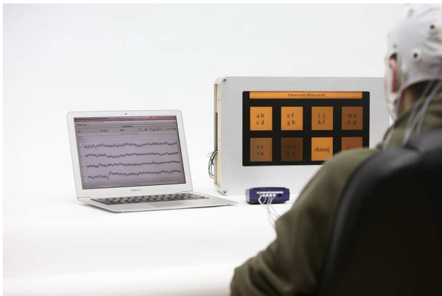
Fig. 3. BCI Appliance running speller; EEG is transferred via bluetooth from the small blue amplifier (5-channel Mobi by TMSI, http://tmsi.com ) to the Appliance (box on the right) running OpenBCI (Sec. 5). Laptop on the left is connected to the Appliance via WiFi, which allows for online display of EEG in the Svarog.pl viewer, connected as an OpenBCI module (Fig. 4)
