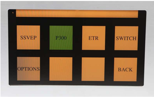
Fig. 5. User-controlled menu of a serial hybrid BCI. Available modes of communication are SSVEP and P300-based BCIs (ERD/S is in the works), eyetracker (ETR) and switch-based interaction. Interface is operating in the fallback SWITCH mode, subsequently highlighting options selectable by a muscular switch
