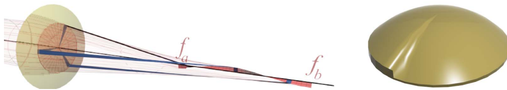
FIGURE 1. (Left) Focusing geometry of the LSL. (Right) Shape of the LSL.
